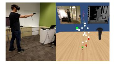
Fig. 2. The physical setup and the corresponding virtual scene as scene from the player's perspective. Green spheres represent the avatar's right hand and ankle while red spheres are the left hand and ankle.
